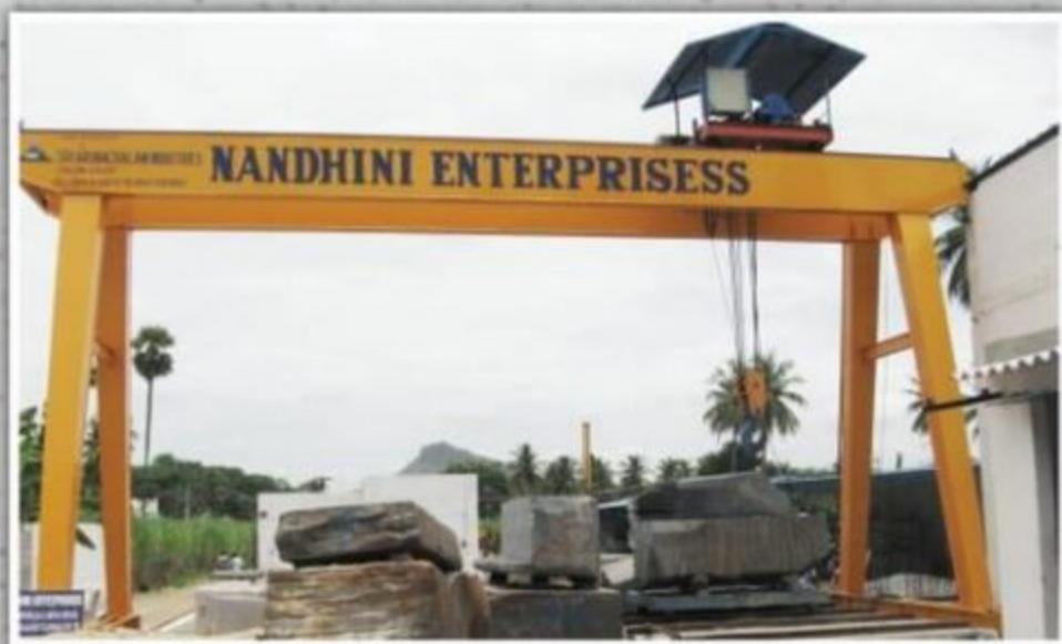
25/40 TONS GANTRY CRANE (MODEL : SAI GC 40,000)
