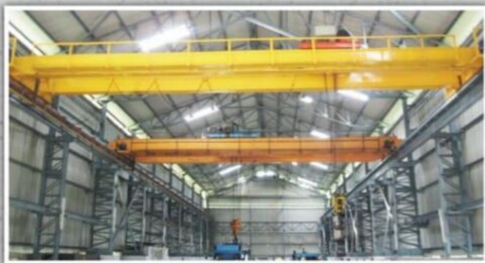
10/15 TONS EOT CRANE (MODEL : SAI E 10,000)
